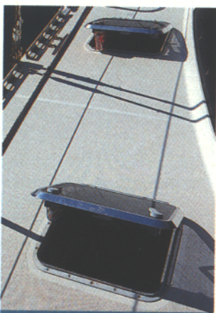
Having someone crack the hatches while you're away from your boat helps keep mold and mildew at bay.
